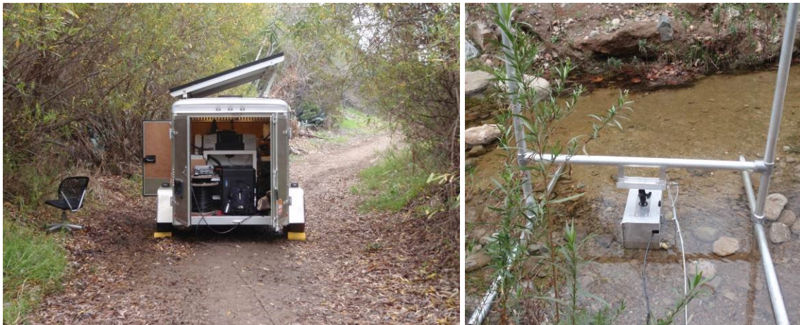
Figure 2: Topanga Creek solar trailer (left), DIDSON in low water (right)
